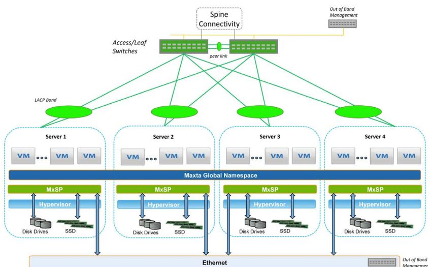
Figure 1: Maxta Storage Platform and Cumulus Networks configuration
